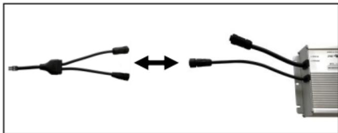
If using the combined power and dimming cable, insert the Pushlock connector into the Power Supply Enclosure's dimming port to power the Dimmer and dim the fixture.
